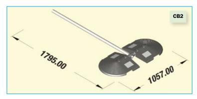
The diagram to the left shows a CB2 counterbalance configuration, for use on free ends when the system has secondary restraint available. Reducing the bay size further can reduce the weight requirement to 1.
